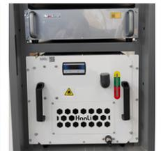
Laser Unit & Thermostatic water tank
